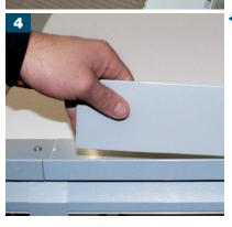
◆ Clip on the BL49 corner section and facing plates to the DP profile, leaving 5mm gap. Clip on connectors to bridge the gap, use multi-purpose adhesive for extra purchase.
