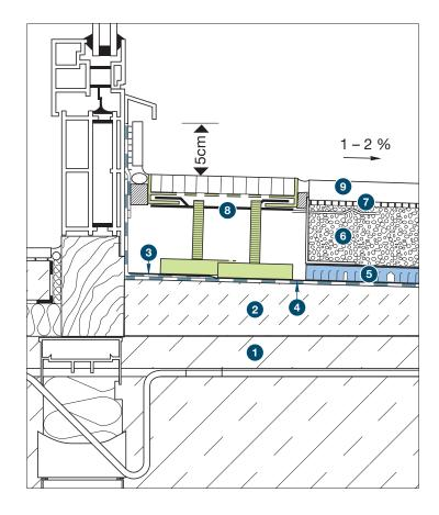
The thick screed assembly with drainage mortar is suitable for most tile types and provides variable height build-up from 68mm. Excellent for use in highly exposed or larger areas, the assembly is typically more cost effective.
