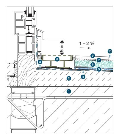
The thin, lightweight assembly with AquaDrain<sup>®</sup> EK drainage mat and MorTec<sup>®</sup> DRAIN epoxy drainage mortar can be used for various tile types and thicknesses. Very strong and lightweight, the build-up can be achieved from only 43mm for low height constructions.
