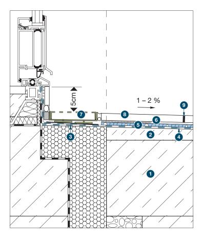
Primarily used for low construction heights and external areas with reduced clearances, this assembly utilises a direct point adhesion method for self-supported breakproof tiles and stone. Recommended for use in areas with limited height, complete construction height can be achieved from 29mm (when using a 20mm slab and 8mm drainage mat).
