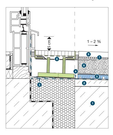
The standard drainage screed assembly with thick screed is suitable for most tile types and provides variable height build-up from 68mm for ground terraces. Excellent for use in highly exposed or larger areas, the assembly is typically more cost effective.
