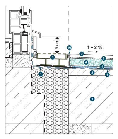
The thin, lightweight assembly with AquaDrain® EK drainage sheets and MorTec® DRAIN epoxy drainage mortar can be used for various tile types and thicknesses. Very strong and lightweight, the build-up can be achieved from only 43mm for low height constructions.
