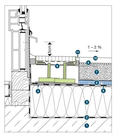
The standard drainage screed assembly with thick screed is suitable for most tile types and provides variable height build-up from 68mm for insulated roof structures. Excellent for use in highly exposed or larger areas, the assembly is typically more cost effective.
