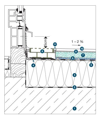
The thin, lightweight assembly with AquaDrain® EK drainage mat and MorTec® DRAIN epoxy drainage screed can be used for various tile types and thicknesses. Very strong and lightweight build-up can be achieved from only 43mm for installation on top of insulated roof structures (insulation >200 k/Pa.)
