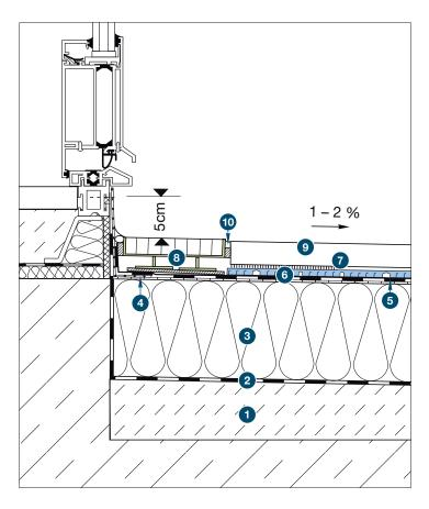
Primarily used for low construction heights and external areas with reduced clearances, this assembly utilises a direct point adhesion method for self-supported breakproof tiles and stone. Recommended for use in areas with limited height, complete construction height can be achieved from 29mm (when using a 20mm slab and 8mm drainage mat).
