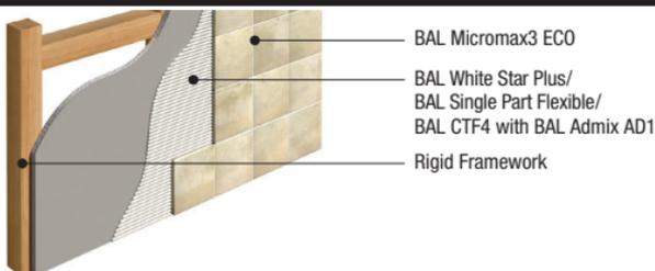
Max. tiling weight: **32kg/m<sup>2</sup>** incl. adhesive and grout
