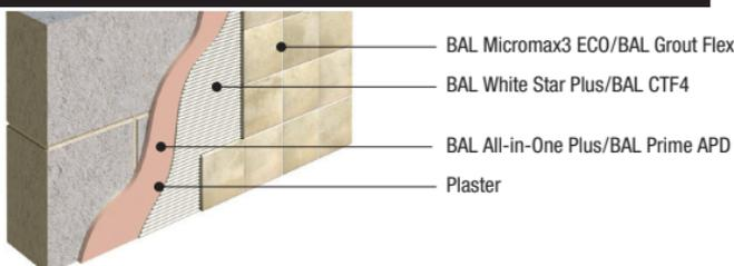
Max. tiling weight: **20kg/m<sup>2</sup>** incl. adhesive and grout
