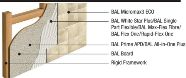
Max. tiling weight (dependent on board type/thickness): **100kg/m<sup>2</sup>** incl. adhesive and grout.
