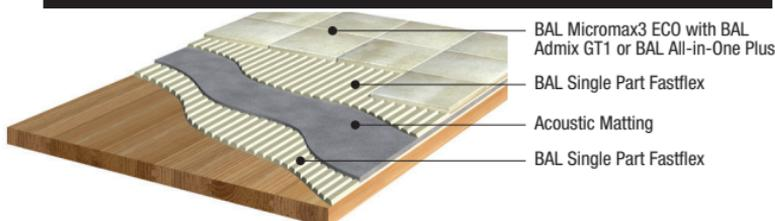
**NOTE:** BAL Single Part Fastflex should be used with approved matting systems to achieve requirements of Building Regulations 2000: Part E – Resistance to the passage of sound.
