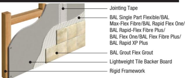
**NOTE:** Check with board manufacturer that tile backer boards are suitable.
